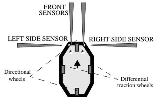
Fig. 3. AURORA's sensing ranges and locomotion.
