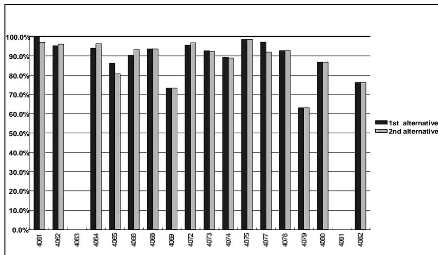
Figure 2: Capacity utilization of assembly stations 4061 - 4082
