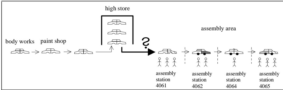
Figure 1: Assembly process of cars
