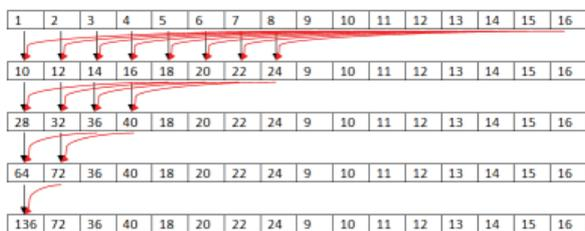
Figure 4: An example of sum reduction. In the first row, eight threads sample two locations in memory, add their values and output the result to a specified location. In the next row, four threads perform the operations. Then, two and one in the final two rows. The total sum is in the first index of the array in the bottom row.
