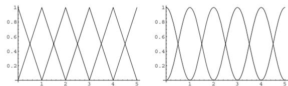
(a) Triangular shaped uniform fuzzy partition (b) Sinusoidal shaped uniform fuzzy partition
