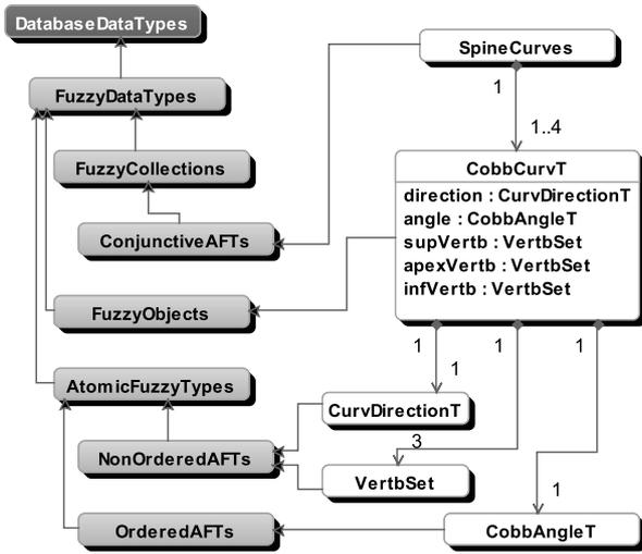
Figure 2: UML Class Diagram for Fuzzy types and SpineCurves Datatype.
