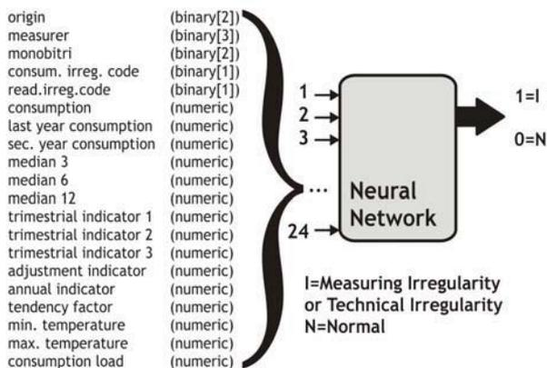
Figure 2: MLP Neural Network topology with one output
