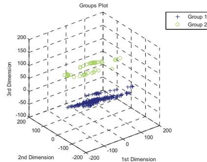
Figure 12: The three-dimensional state space representation of the Visbreaker process in the last week of May and the first week of June 2008. Blue points are normal operating point. Group 2 are points of a simulated sensor malfunction situation.
