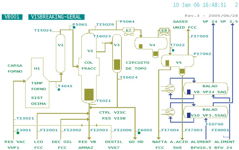
Figure 8: The Visbreaker Process [10].
