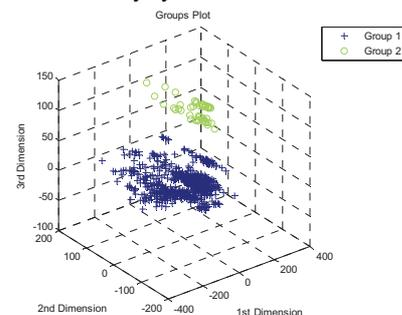
Figure 15: The three-dimensional state space representation of the Visbreaker process during the 5<sup>th</sup> of May and the 5<sup>th</sup> of June 2008. Blue points are normal operating point. Group 2 are points of a simulated sensor malfunction situation.
