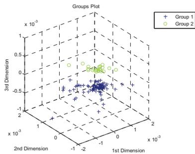
Figure 9. The three-dimensional state space for Case 1. Blue points (Group 1) are normal operating point. Group 2 are points of a simulated sensor fault.
