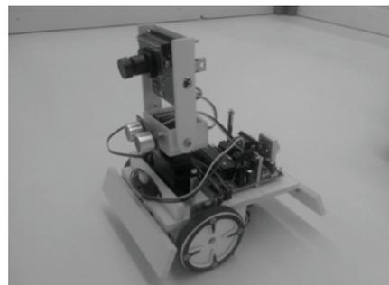
Figure 1. The real box-pushing robot
