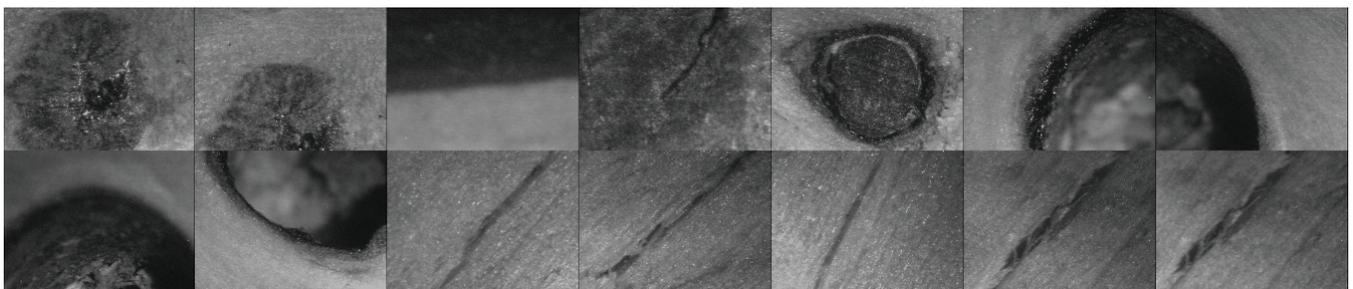
Figure 4: Images of wood with knot defect and other wood irregularities
