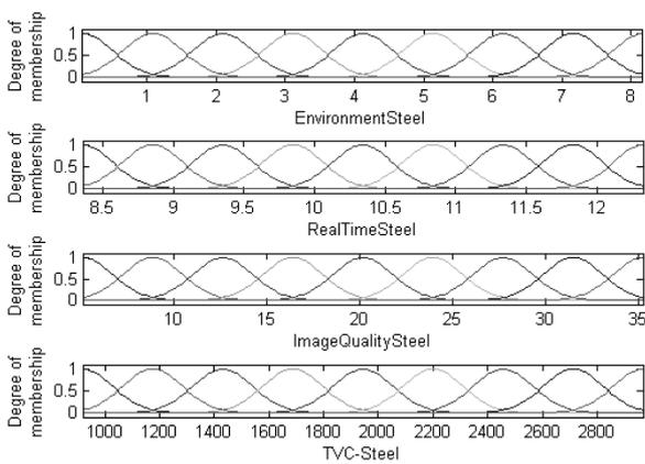
Figure 9: Membership functions with 9 nodes for E, IQ, RT and CVT parameters on Stainless Steel images.
