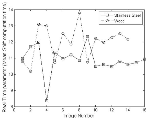
Figure 6: Evolution of the Mean-Shift computation time in Stainless Steel and Wood images.
