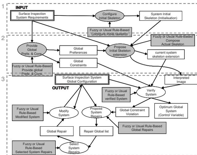
Figure 1: Subtask and inference diagram of the method Propose-&-Revise to solve the surface inspection task.
