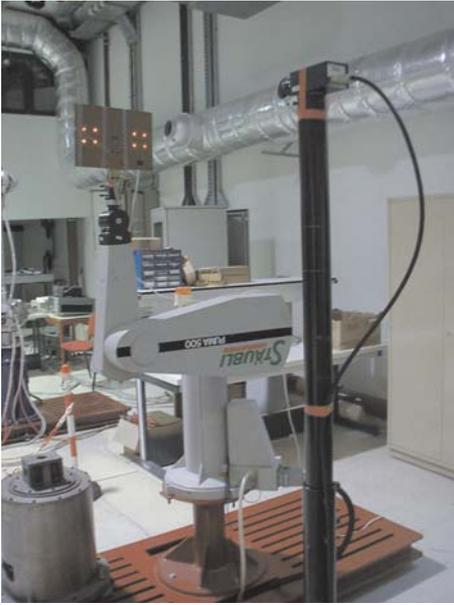
Figure 1: The eye-to-hand experimental setup.
