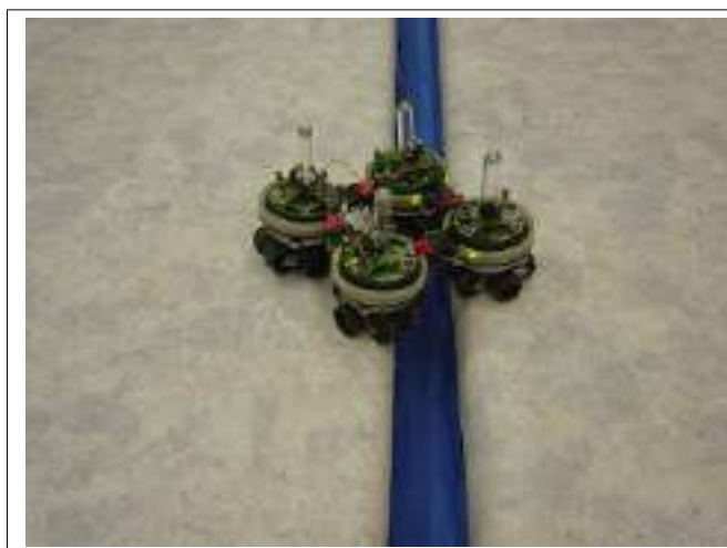
Fig.2 A swarm-bot made of four s-bots attached to each other can pass over a trough that is too large for a single s-bot.
